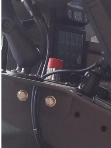
< Emergency stop switches >
