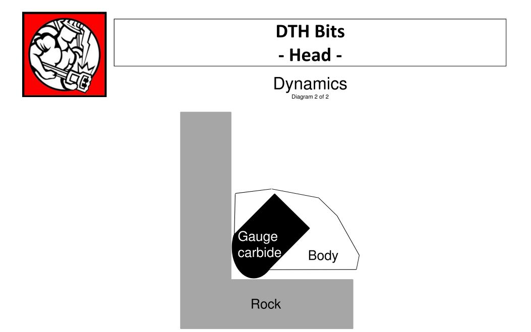
As the carbide buttons starts to wear, they develop a flat surface. As the flat enlarges the load on the carbide changes from compressive to shear.
