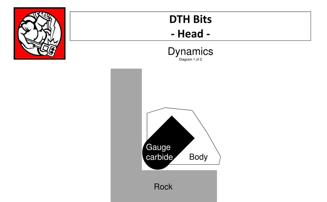
Carbide buttons are designed to resist compressive forces not shear forces.
