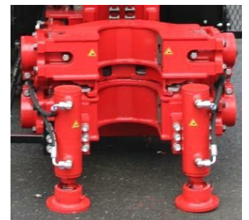
Double rod clamp with casing extraction jacks
