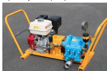
Triplex injection pump
