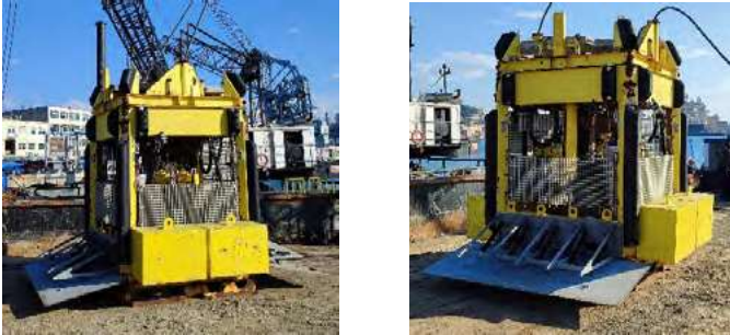
Figure 4. setup of the equipment and MANTA Penetrometer
